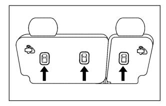
Do not secure a child restraint in the right front passenger's position if a national or local law requires that the top tether be attached, or if the instructions that come with the child restraint say that the top tether must be attached. There is no place to attach the top tether in this position.
